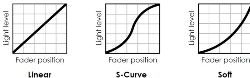
**Figure 2. Dimming curves**
