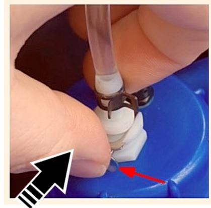
**Figure 10. Releasing the disinfectant tube**
