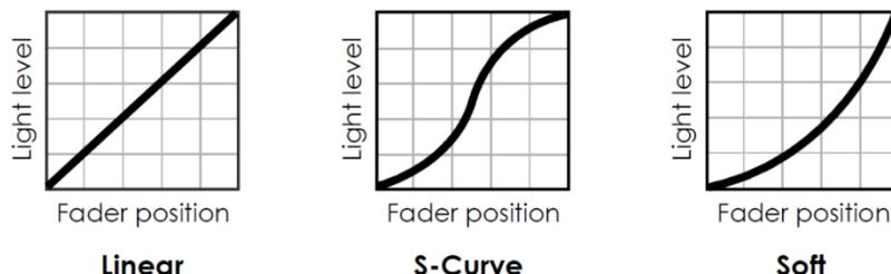
**Figure 2. Dimming curves**
