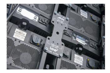
Figure 7. KNV Multi Connector Plate
