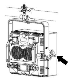
Figure 13. Single KNV Cube suspended in Floorstand-Bracket
