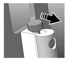
Figure 12. Safety latch on Installation Bracket
