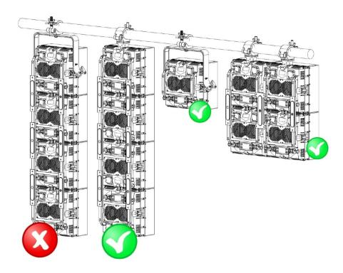
Figure 15. Installation hardware for suspending multiple fixtures
