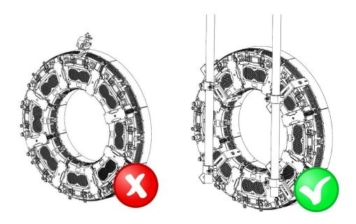
Figure 18. Supporting a circular array of KNV Arcs
