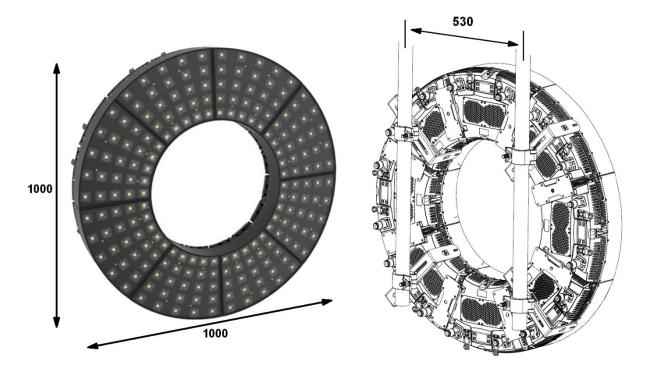
Figure 16. KNV Arc circular array dimensions
