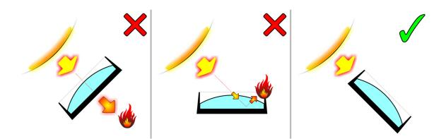
Figure 1. Avoiding damage from light sources
