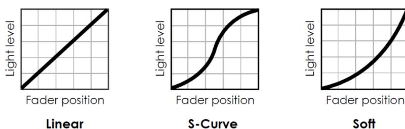
**Figure 2. Dimming curves**
