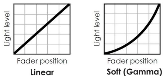
Figure 7. Dimming curves
