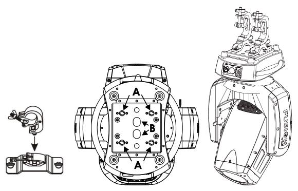
Figure 4. Omega bracket fasteners
