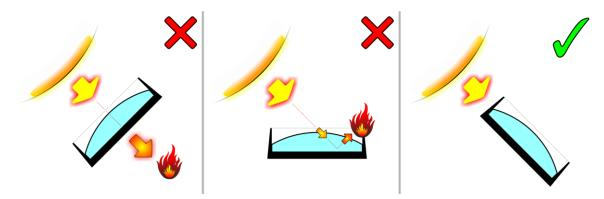
Figure 1. Avoiding damage from light sources
