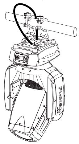
Figure 3. Safety cable attachment
