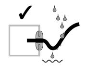
cable slack and create 'drip loops' before connectors.
