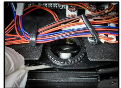
**Figure 15. Removing a glass gobo**
