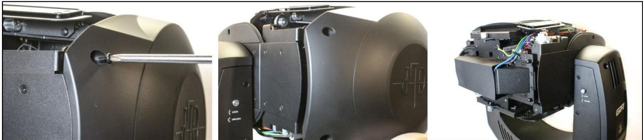
**Figure 14. Rear head cover removal**
