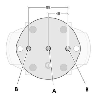
Figure 5. Mounting points in base
