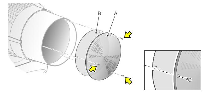
Figure 9. Removing a micro-Fresnel lens
