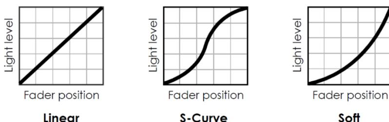
**Figure 2. Dimming curves**
